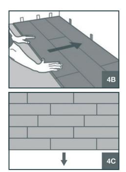
Always ensure that the end joints are randomly staggered at least 400mm apart.
