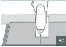
Always ensure that the end joints are randomly staggered at least 400mm apart.
