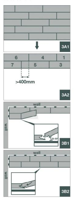
You can tap the long side of the plank into the groove by using a professional tapping block. The planks should not be joined by a single tap. To avoid damaging the planks, you must tap them together gradually.
