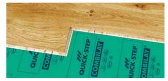
Quiet • Step® Combi-Lay is a superior underlay, where reduced reflected foot noise and sound reduction in multi- story buildings are required. It is made of high density polyolefin copolymer resin which effectively reduces the hollow and often "clunky" foot noise associated with floating floors. Quiet • Step® Combi-Lay addresses this key negative of floating floor installations, while performing all the tasks of a superior quality underlay including a continuous damp proof\*.
