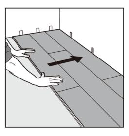
**8.** To lay the last row: position a loose board exactly on top of the last row laid. Place another board on top, with the tongue side touching the wall. Draw a line along the edge of this boards, to mark the first board. Cut along the edge of this board to mark the first board. Cut along this line to obtain of the required width. Insert this cut board against the wall. The last row should be at least 50mm wide. The spacers can then be removed.
