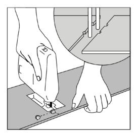
**10.** Architraves and skirting: lay a board (with the decorative side down) next to the architrave as shown in the figure. Under-cut the architrave and door jamb, allowing 1mm gap between AquaPlank and underside of the jamb. Then slide the floorboard under door frame.
