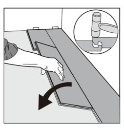
**7.** After 2-3 rows. Adjust the distance to the front wall by leaving an expansion gap of 10mm. Always ensure that the end joints are staggered at least 30cm, both when in the same row as when from one row to the next one.
