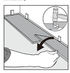
**3.** At the end of the first row, leave an expansion gap of 10mm to the wall and measure the length of the last plank to fit.
