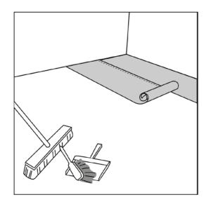
**2.** Begin laying in the left-hand corner. Place the floorboard 10mm from the left wall. Use spacers between the wall and the floorboard.
