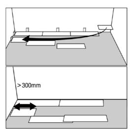
**6.** Click the long side of the plank into the previous row and place it tight to the short end of the previous plank.
